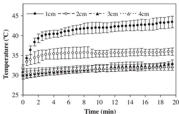
Fig. 8. The mean  $\pm$  SD of temperature changes (°C) at different depths in mice (1, 2, 3 and 4 cm) versus duration of sonication (min) under dual frequency sonication conditions (3 MHz and 28 kHz).
