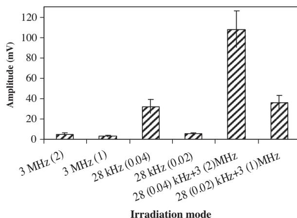
Fig. 6. Signal amplitudes (mV) at 14 kHz (a subharmonic of 28 kHz) of the 28 kHz and 3 MHz sources applied alone and in combination and presented as mean  $\pm$  SD. The background has been subtracted from all values. The values in the parentheses are intensities in  $\text{W/cm}^2$ .
