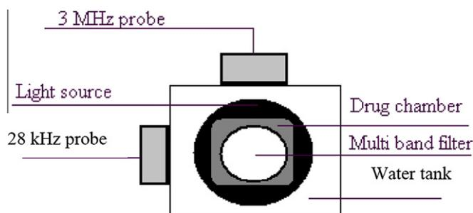
Fig. 2. Setup for the measurement of doxorubicin release *in vitro*. Elements include the 3-MHz probe, the 28-kHz probe, the filter on which the camera was mounted, the light source that is placed at the bottom and the drug chamber that was placed in the water box on the light source.
