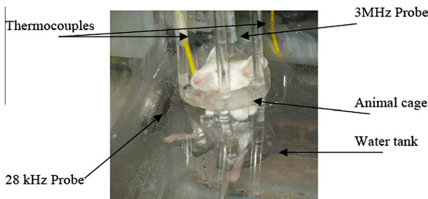
Fig. 3. Animal sonication setup. A side view of the animal cage in the sonication condition. The 28-kHz probe, 3-MHz probe and thermocouples are shown.
